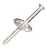
The type W clip is used to secure GLOBALGRID mini-mesh grating to the substructure. It is made of stainless steel. One set of clip includes W clip and self screw bolt, and it is easy installed with a hand electric drill and screwdriver.
